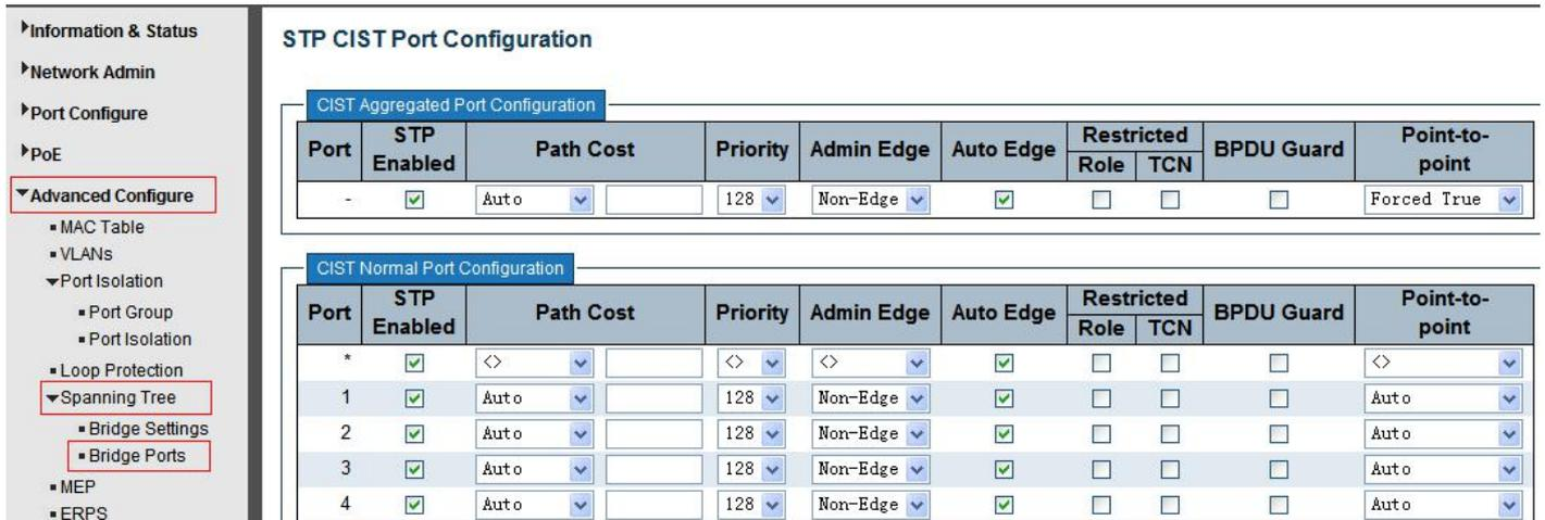
Figure 5-5 STPConfiguration Screen
