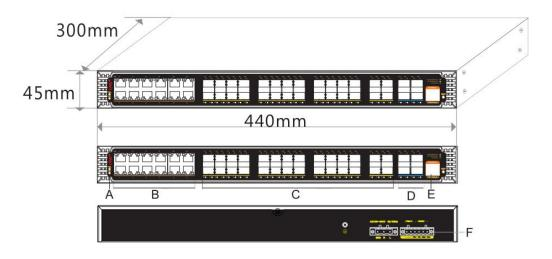
A.Power indicator C.28\*Gigabit SFP ports E.Console port B. 12\* RJ45 Ports D.4\*1/10G SFP Ports F.AC/DC dual input port
