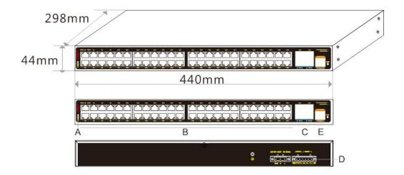
A. Working indicator B. 48\* RJ45 ports
